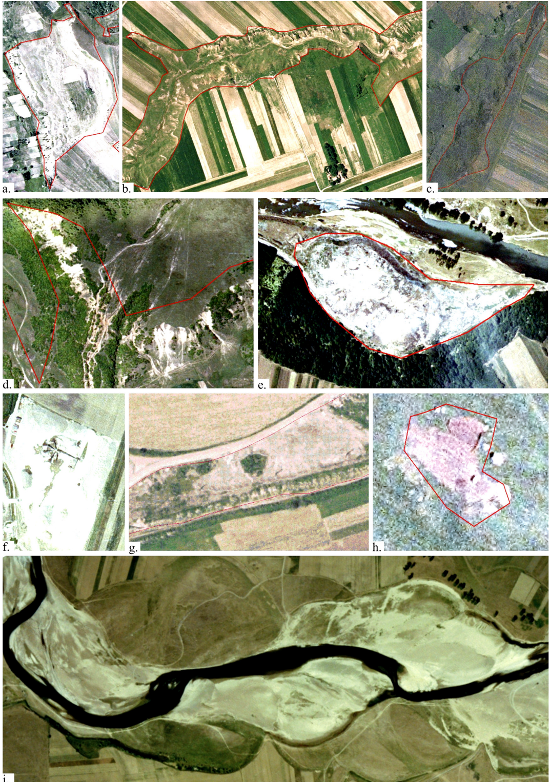
Fig. 1. Soil damage forms taken into account: a. wide area soil erosion; b. gully erosion; c. landslide; d. landslide with terrain collapsing processes; e. garbage deposits; f. gravel deposits; g. artificial land slopes; h. overgrazed zones; i. major waterbed of the Suceava River, with land movement phenomena present.
